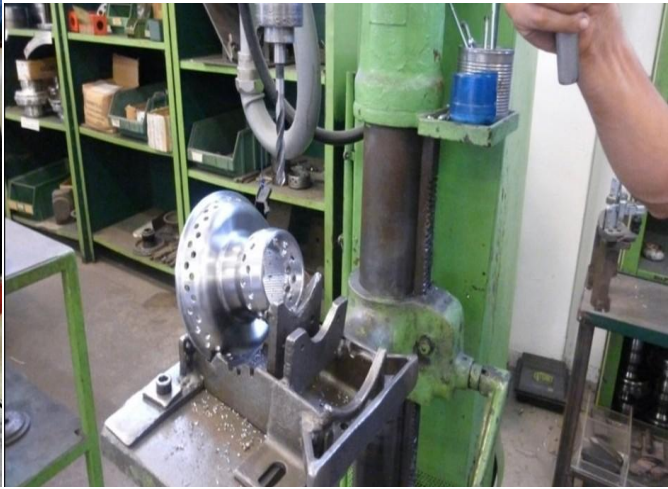
Spline Hub Drilling
