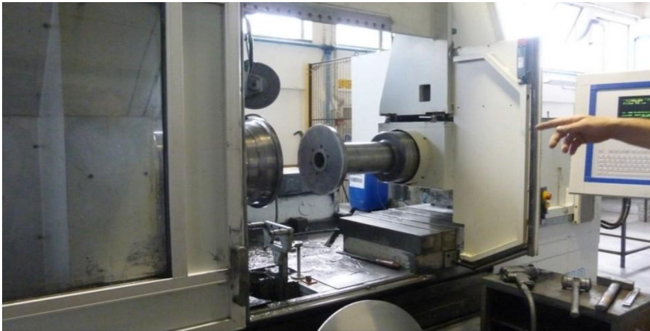
Spinning a rim from an alloy disc of silicone and magnesium alloy -computerised machine.
