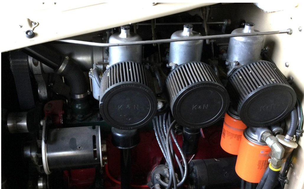
Supercharged highly modified flat 6 engine, Triple SU Carbies.,6500 RPM Capable of 160 MPH. Suspension and tyre mods. Holden Body - body restoration and paint by Chris
