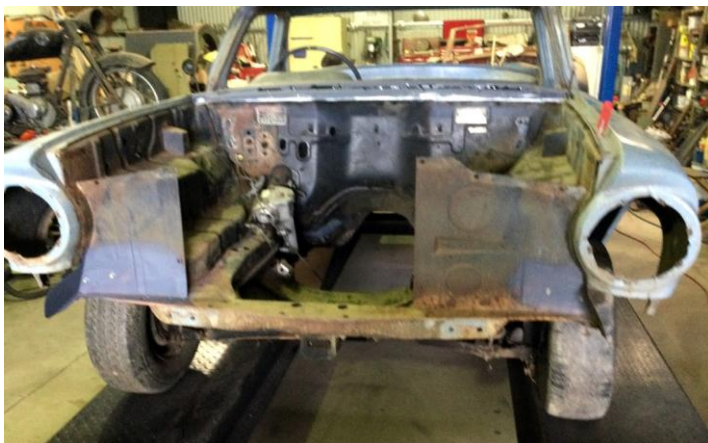
Holden EJ Ute - Rust replacement metal fabrication
